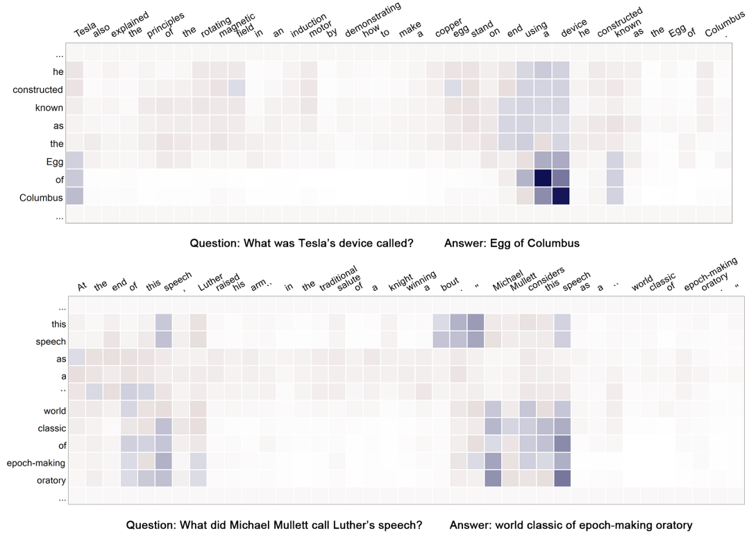
Figure 2: Part of the attention matrices for self-matching. Each row is the attention weights of the whole passage for the current passage word. The darker the color is the higher the weight is. Some key evidence relevant to the question-passage tuple is more encoded into answer candidates.
